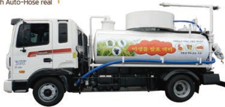
오토호스릴 장착 4x2 액비살포차 4x2 Liquid Fertilizer Sprayer with Auto-Hose reel
