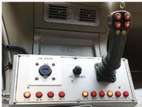
3-Stage waterproof control device & Bumper waterproof gun panel 3단방수 제어장치 & 범버 방수총 판넬
