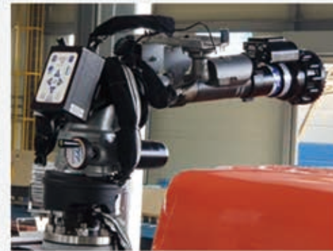
Automatic waterproof gun & Nozzle 자동방수총 & 노즐
